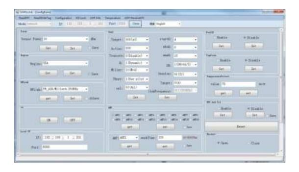
After device has connected with PC, the parameters on interface will be empty. Click "Get" on each option to collect device parameters.
