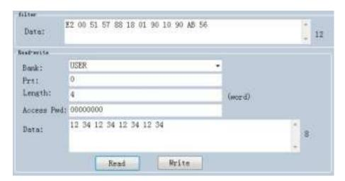
Data could be written in EPC, RESERVED and USER areas, select according areas and input initial address, length, input data into "Data" window and click "Write" to write data into according areas.
