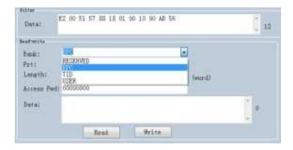
Click one option in "Read-write" window to enter tag reading mode, EPC will be automatically copied into "Data" block in filter, default option is EPC reading, click "Read" to read 12 bytes of EPC area.
