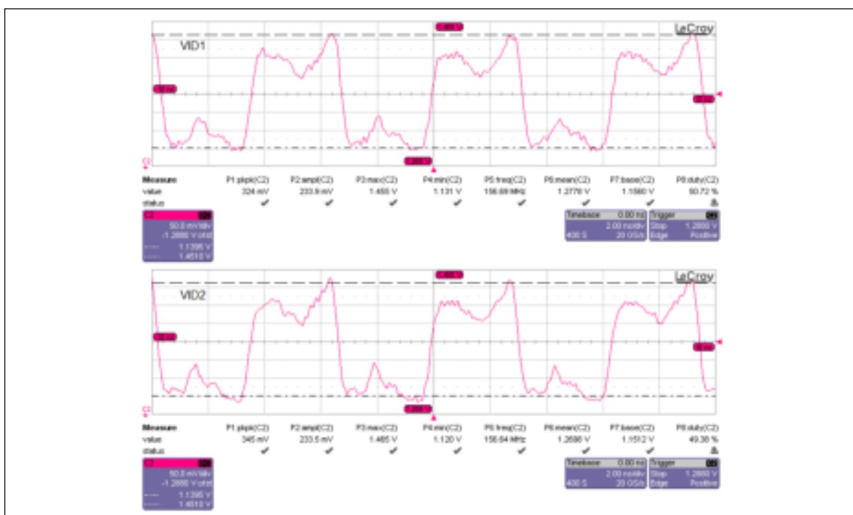
FIGURE 3: Measured Waveforms, LVDS to LVDS25_ODT, Direct Interface (Waveforms Measured on RTG4 DevKit).
