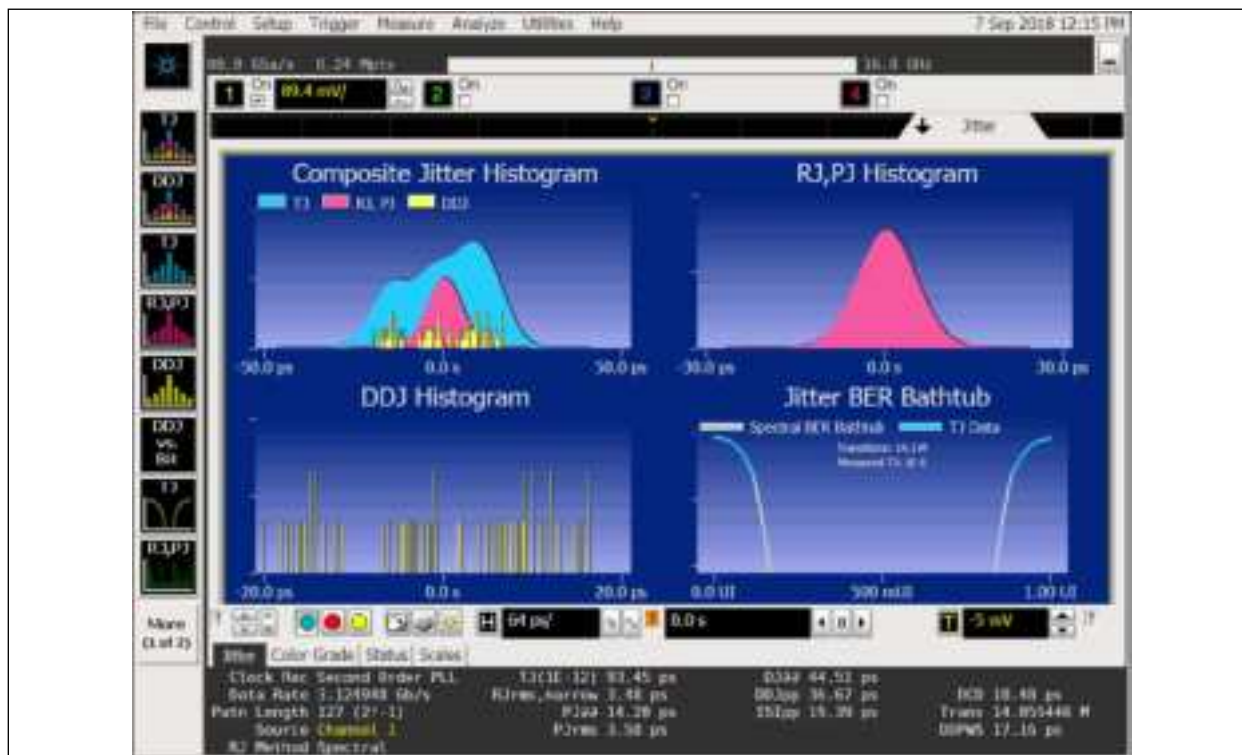
FIGURE 17: Jitter Data, LVDS to LVDS25 200Ω External Termination (Setup Figure 4).
