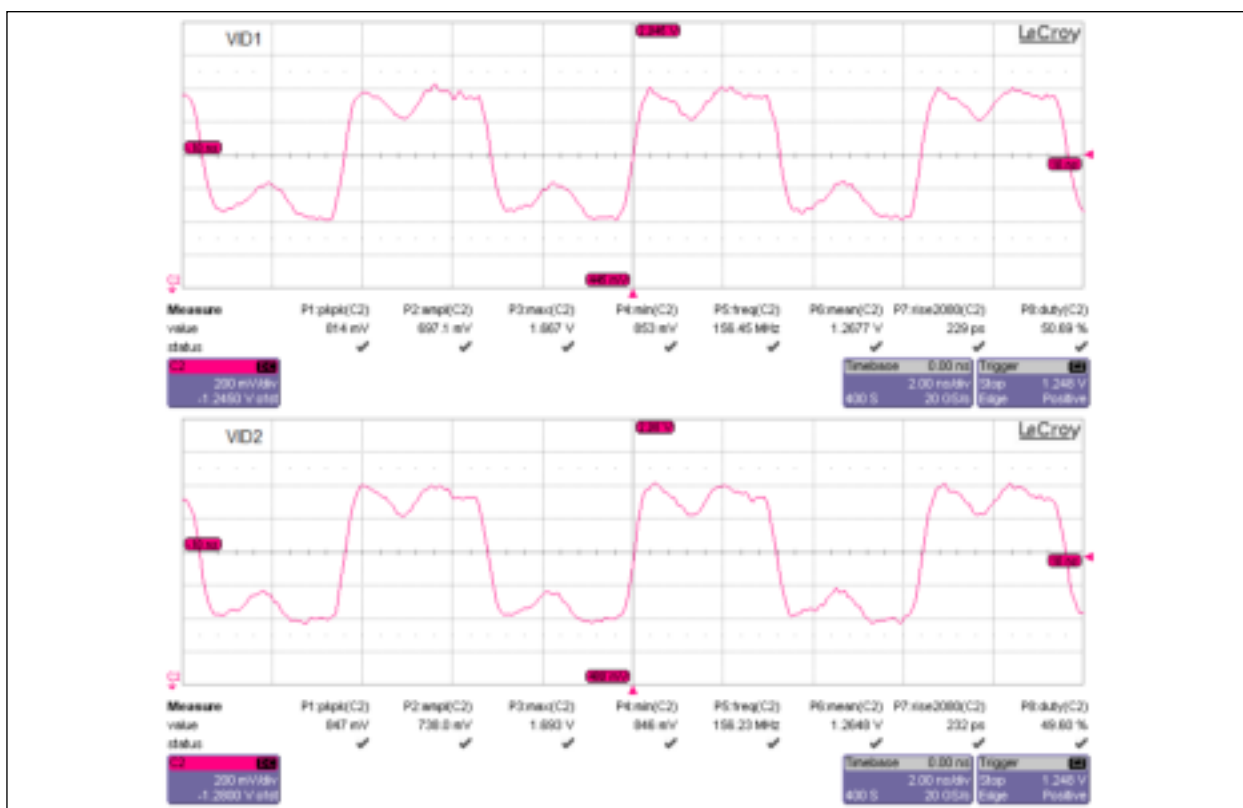
FIGURE 8: Measured Waveforms, LVPECL to LVDS25_ODT, V_{ICM} 3.3V-Bias (Waveforms Measured on RTG4 DevKit).
