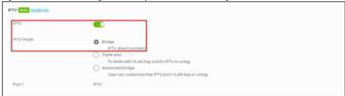
Figure 141 Site-wide > Configure > Security router > Interface: Bridge Mode
