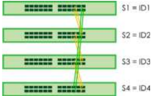
Figure 116 Onsite Stacking Cable Connection: Ring Topology
