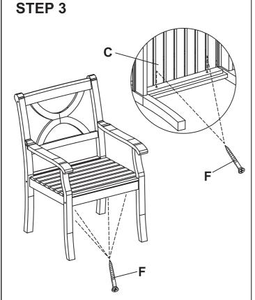
Next, secure the seat (C) using 1" screws (F).
