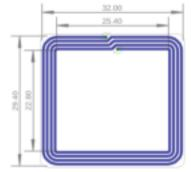
HF antenna on external PCB, printed, one-sided
