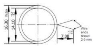
LF antenna on external PCB, glued and soldered
