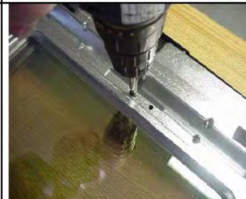
Unscrew the two screws located on the left and right side of the glass
