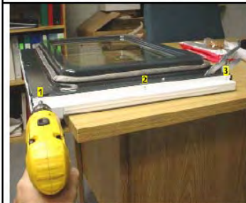
Unscrew the three screws from both the left and right hand side door trim
