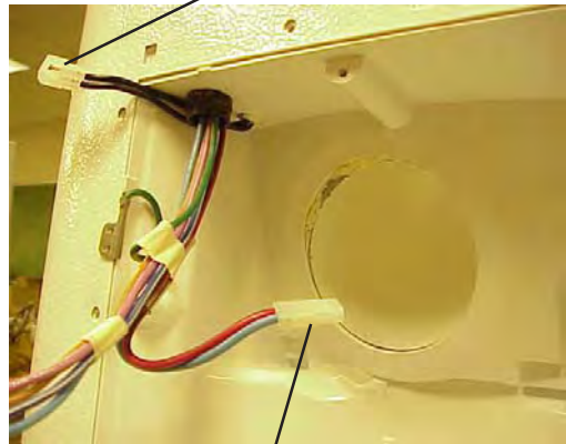
Plug for chute heater Figure 26
