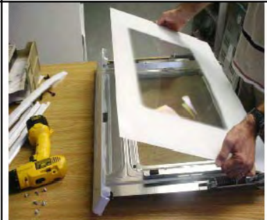
Remove the outer door glass
