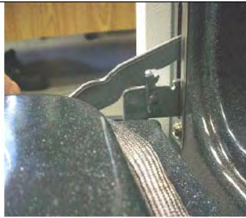
Door hinge in the lock position
