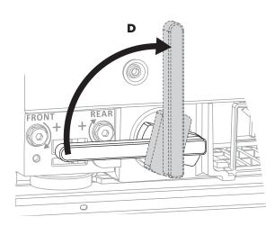
(§) Rotate the filter head clockwise 90° to lock in place (**D**).
