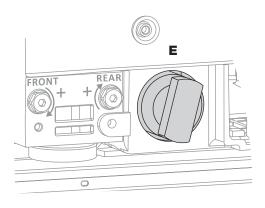
⑤ Ensure the filter is in the locked position (E). Remove filter removal tool and close the freezer drawer.
