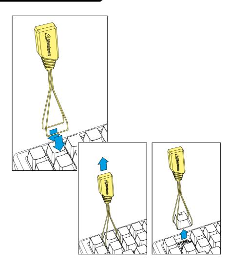
Before removing a switch, first remove the keycap. To do this, place the arms of the keycap puller tool either to the left and right or to the top and bottom of the keycap, and then pull the keycap upwards with careful but constant pressure. Whenever possible, avoid pulling the keycaps from the switch directly with your fingers, as this may damage the switch.
