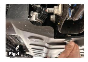
Step 3. Disengage the inserts that secure the air deflector under the charge air coolant heat exchanger bottom bracket. This will allow for the heat exchanger removal in later steps.
