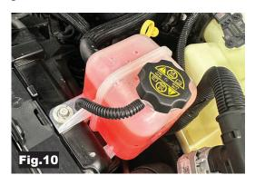
Step 18.Drive truck for at least 15-20 minutes to purge the air in the charge air coolant loop, then top off coolant to the factory recommended fill level again.
