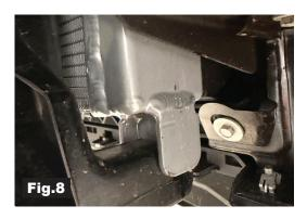
Step 15. Reconnect the inlet and outlet hoses, reengage both clamps.
