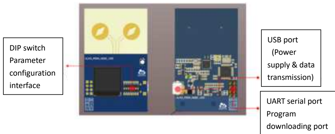
Figure 5-1 Module Interfaces
