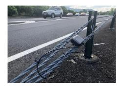
The Viotel Smart Barrier node features a unique patented design for quick installation on wire rope barriers and fences. The node measures the tension of the wires, and monitors the barrier for impacts.
