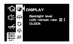
Higher refresh rate provide more smooth LCD viewing experience but it consume more battery. How to adjust LCD refresh rate level. When you spot the LCD refresh rate setting, click the upper ■ to select backlight setting. Then click ▲ or ▼ buttons to increase or decrease the LCD refresh rate.
