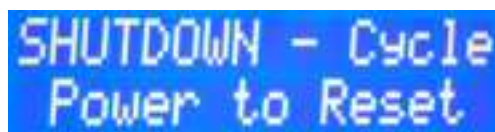
Figure 6-3 LC-display when Emergency Shutdown button is pressed
