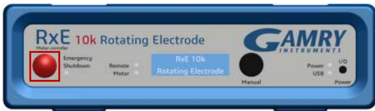
Figure 4-9 Emergency Shutdown button of the Motor Controller
