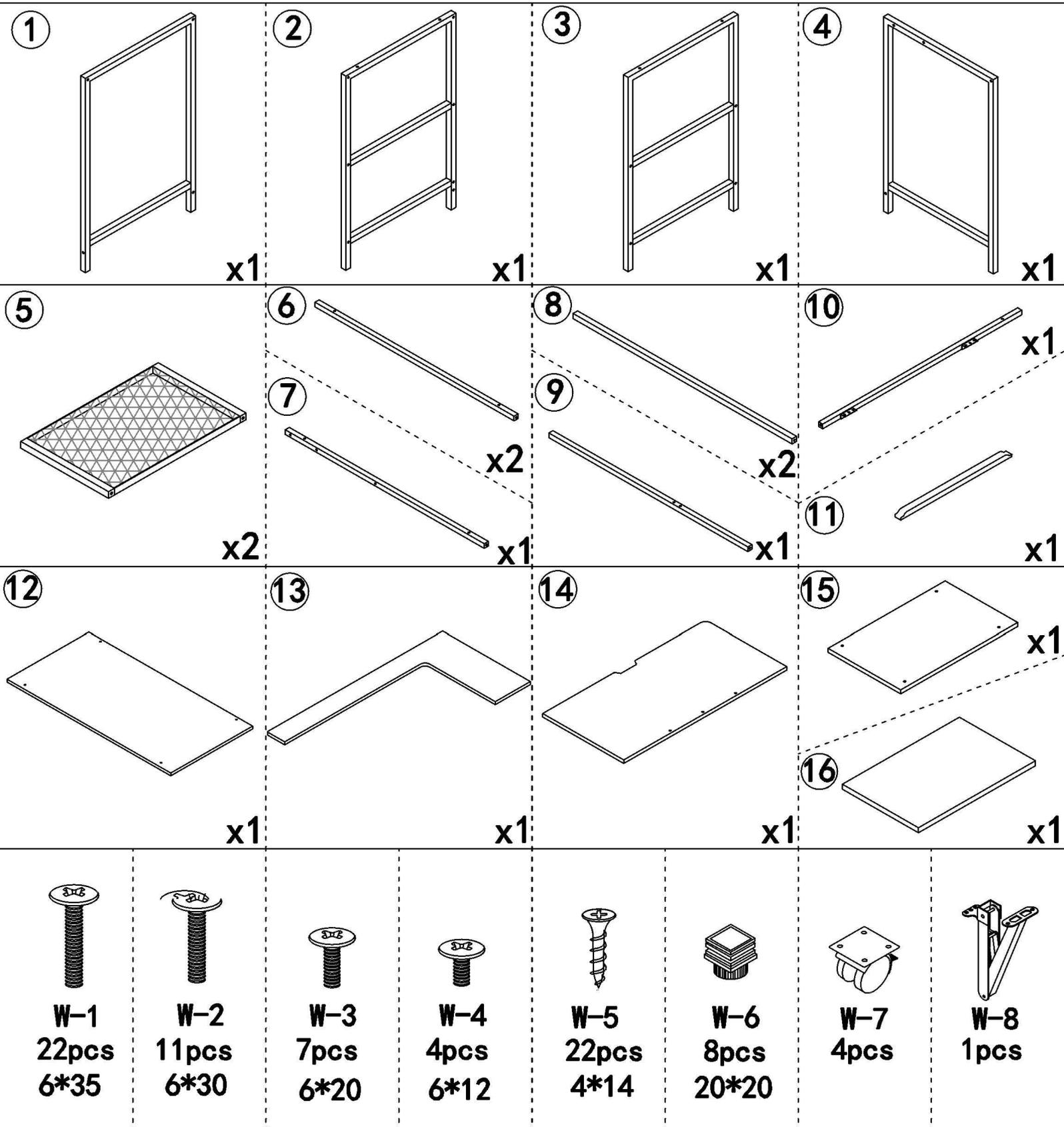
**NOTES:** Don't tighten screws completely at first, just in case parts were assembled wrong and need disassembled. Tighten screws at last when all parts are put together.
