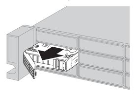
${f 3}$  Insert the new drive into the empty slot with the lock mechanism remaining open.
