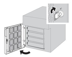
$\boldsymbol{2}$  Remove the front cover while holding the hook downward.
