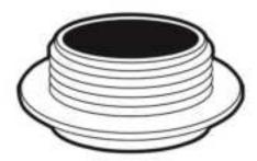
Connect the network cable, fiber-optic jumper, and AC power cable to the AP after they pass through the corresponding waterproof plugs to ensure waterproof.
