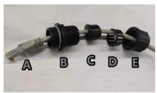
Figure 3-10 Passing the Network Cable Through the Waterproof PG Connector
