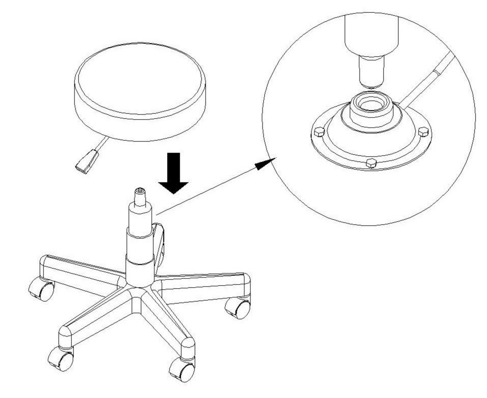
1.Align the top of the gas lift with the center hole on the underside of the seat cushion, then press down to attach the cushion.
