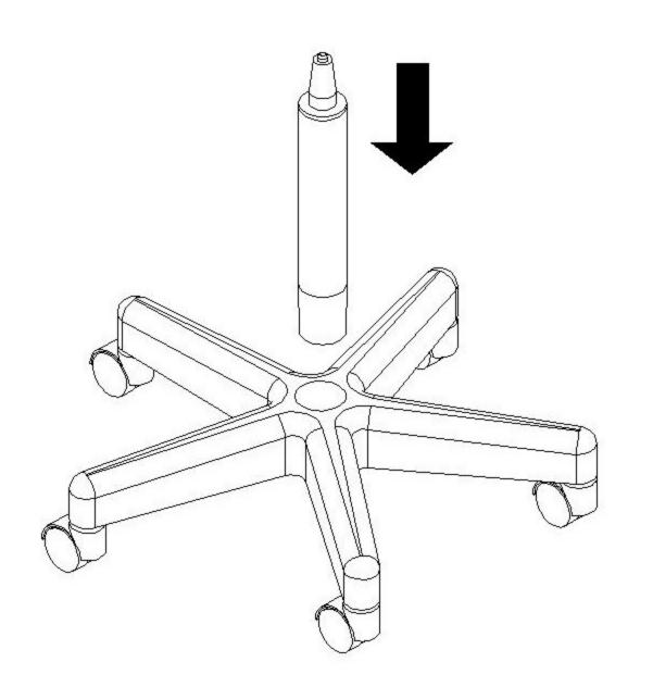
1.Insert the gas lift into the stool base, ensuring the larger end is pointing downward.
