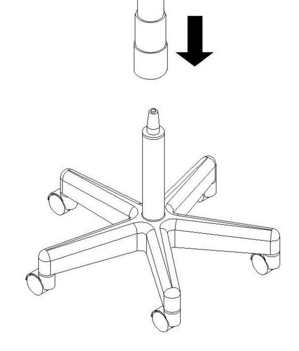
1. Carefully slide the protective cover over the gas lift from the top until it is fully secure.
