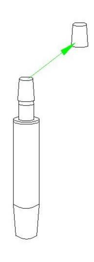
1.Remove the protective black plastic cap from the gas lift and discard after removal.
