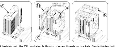
Put heatsink onto the CPU and align both nuts to screw threads on brackets. Gently tighten both nuts with screw driver to install heatsink on CPU.Install both fan with fan wires, and be aware of airflow direction. Align LCD install position to heatsink screws, put LCD cover on top of heatsink.
