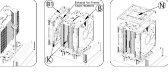
Put heatsink onto the CPU and align both nuts to screw threads on brackets. Gently tighten both nuts with screw driver to install heatsink on CPU.Install both fan with fan wires, and be aware of airflow direction. Align LCD install position to heatsink screws, put LCD cover on top of heatsink.
