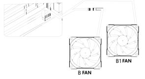
For Fans with Addressable-RGB lighting, connect 3-Pin ARGB lighting header to motherboard 3-Pin +5V ARGB lighting socket to control lighting effect.
