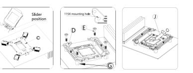
Push slider on backplate to 115X hole position. Install backplate from back side of motherboard. Put 115X/1200 spacers onto backplate screw threads, then fix both brackets on spacers with intel screws.Apply thermal paste on CPU IHS.
