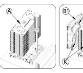
Put heatsink onto the CPU and align both nuts to screw threads on brackets. Gently tighten both nuts with screw driver to install heatsink on CPU.Install both fan with fan wires, and be aware of airflow direction. Align LCD install position to heatsink screws, put LCD cover on top of heatsink.
