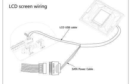
1.LCD is powered by connecting SATA power connector. Data is transmitted by motherboard USB connector. Please confirm proper connection before software install.
