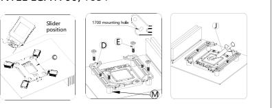
Pull slider on backplate to 1700 hole position. Install backplate from back side of motherboard. Put 1700 spacers onto backplate screw threads, then fix both brackets on spacers with intel screws. Apply thermal paste on CPU IHS.
