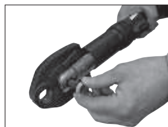
Figure 4 — Pushing and twisting to open the jaw set mounting pin
