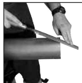
Figure 4: Deburr outside diameter using a half-round file
