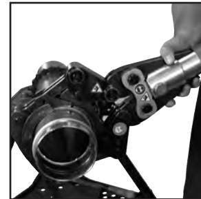
Figure 8: Placement of adapter jaw into pressing chain
