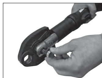
Figure 4 — Pushing and twisting to open the jaw set mounting pin
