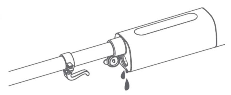
**NOTE:** The water tank should be emptied after each use to prevent mineral build-up and overfilling.
