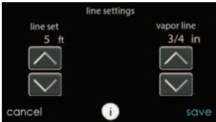
Fig. 18 – Adjust Line Set Length &amp; Vapor Line Diameter that is Installed
