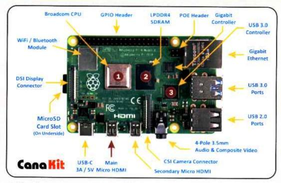
1. If you have a case, start by installing the Raspberry Pi inside the case. To avoid damaging your MicroSD card, do NOT insert the card until the board is installed in the case. You can find video instructions for CanaKit cases at:
