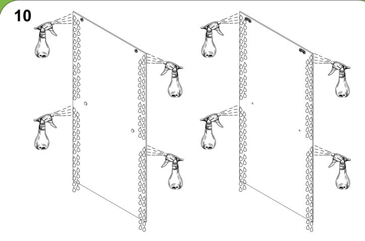
Spray water on both sides of the glass for easy installation of rubber strips.
