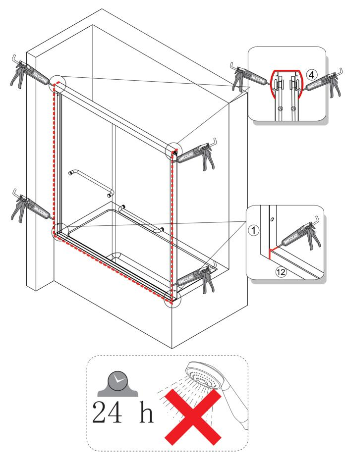
Do not use the shower enclosure for at least 24 hours in order to allow the silicone sealant to cure fully.
