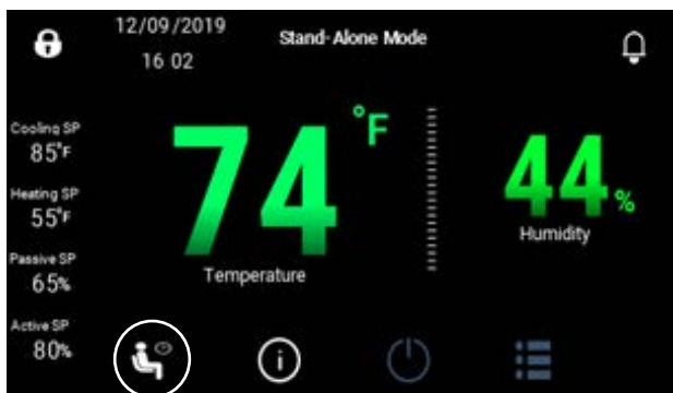
FIGURE 36 Accessing Comfort Mode via Main Screen
