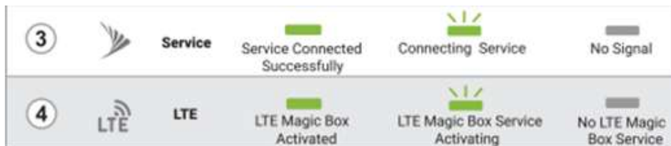
Figure 4: Sprint Magic Box Silver- LTE activated LED status
