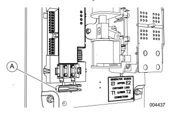
Figure 4-2. Fuse Removal and Installation Tool
