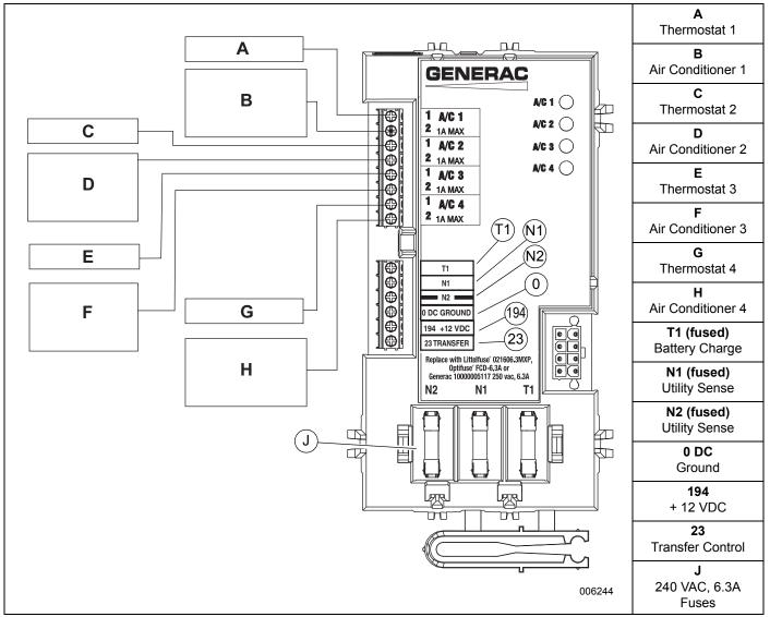
Figure 3-3. Typical SACM Connections
