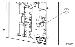
Figure 3-4. Auxiliary Contact
