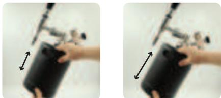
Repeat step 10, in our practice, one good N2O cartridge can dispense all coffee liquid out at once. If you think the coffee is not good cascading effect or the pressure on gauge is a little low, you can fill 2nd cartridge, and then shake for a while, and then pour.
