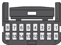
AUXILIARY CONNECTOR (16 PIN) REAR VIEW (WIRE SIDE)
