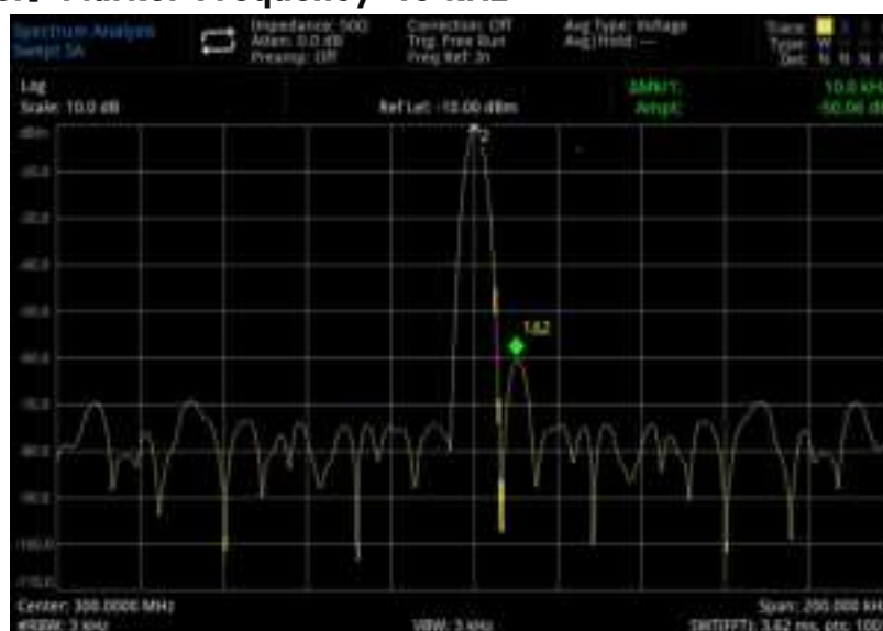
Figure 3-9: Distinguish Small Signal from Big Signal
