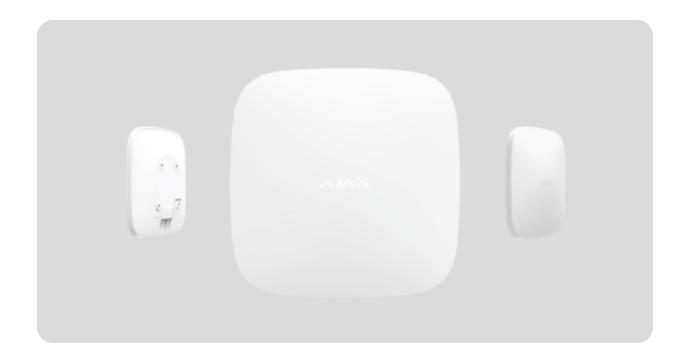
**ReX Jeweller** is a range extender of communication signals that expands the radio communication range of Ajax devices fitted with a hub up to 2 times. Developed only for indoor use. It has a built-in tamper resistance and is equipped with a battery that provides up to 35 hours of operation without external power.
