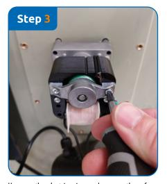
Unscrew the electric wires and remove them from the terminal block (**Photo step 2**). Then unscrewthe ground wire (**Photo step 3**) and put the cover with the wires stuck in it to one side.
