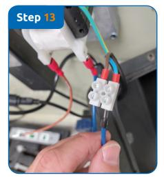
Attach the supplied cable shoes over the contacts on the motor (it does not matter where the brown and blue wire are, Photo step 12) and screw them back into the terminal block (Photo step 13).
