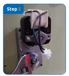
If the white coil is down, it is difficult to reach the locknut of the shaft. To have good access to it, completely loosen the 2 boltsholding the coil (**Photo step 3**) so that you can remove the coil completely. As you replace the complete motor, there is no need for keeping the coil on.
