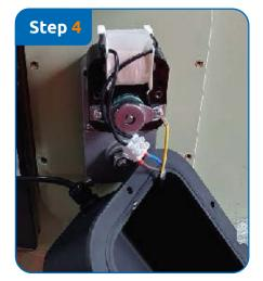
Now there are 2 options regarding the position in which the motor is mounted: if the white coilis up as in photo 4, then continue with step 6. If the white coil is down as in photo 3, then continue with step 5.
