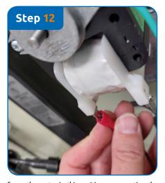
Screw the motor in this position, reconnecting the ground wire (Photo step 11).
