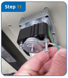
Then loosen the two screws on the new motor (Photo step 9) and turn the motor 180° so that the coil is pointing down again (Photo step 10). Make sure that the black ring in this block remains in the right place.
