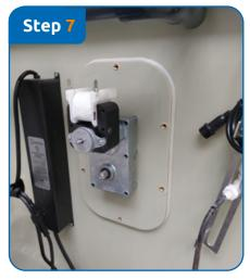
Now loosen the bolts holding the motor to the filter (Photo step 6).
