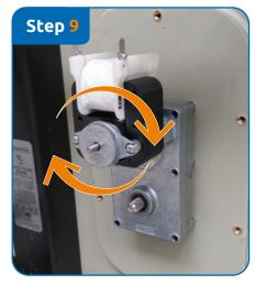
Now place the new motor over the shaft (Photo step 7) and screw the motor back to the filter wall with the hex head bolts as it was (Photo step 6)
