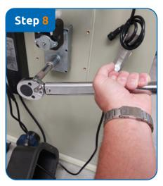
Remove the locknut completely and carefully remove the motor from the shaft. Make sure that the seal ring around the shaft does not fall and you lose it.
