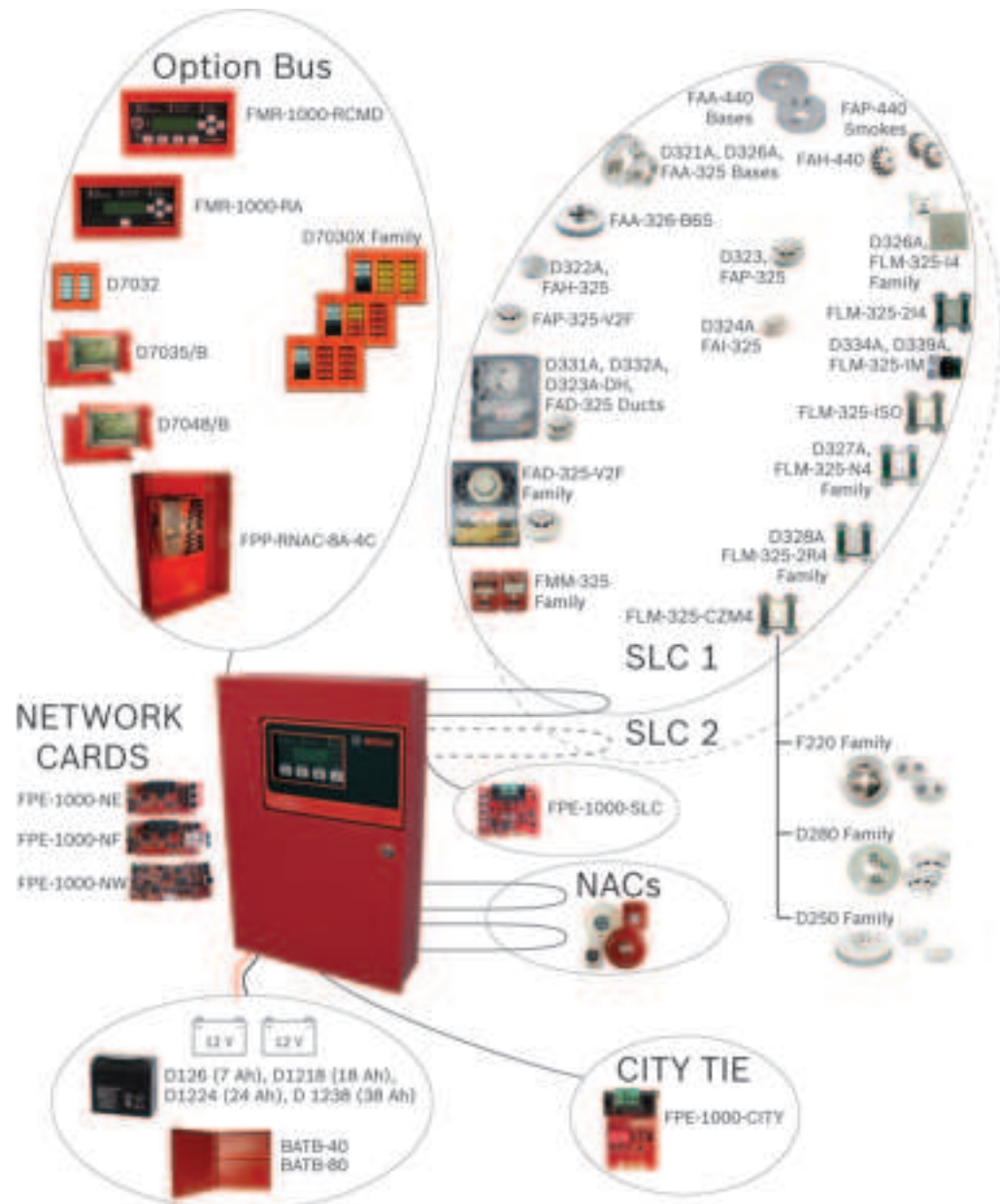
Figure 2.1: FPA-1000-V2 System architecture
