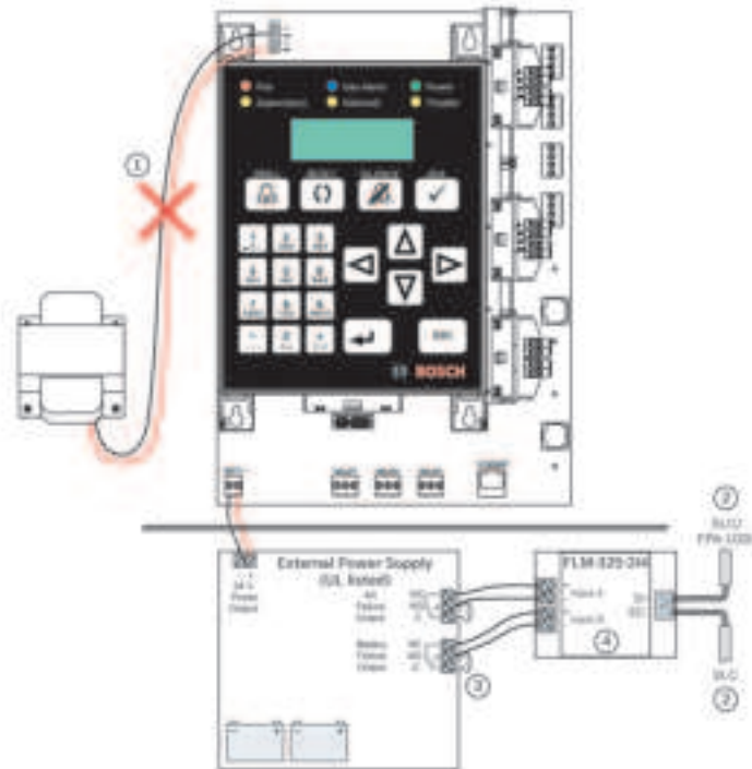
Figure 4.26: Connecting external power supply & Dual input monitoring module
