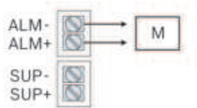
Figure 4.10: City Tie wiring in reverse polarity mode
