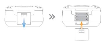
Open the battery cover on the back of the transmitter. Put in three AAA batteries (not included). Then, close the cover.
