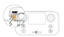
**Take photo:** Short press the button. The transmitter will beep once, and the icon on the LCD screen will flash once. The camera will take one picture.
