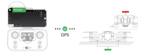
After calibrating the compass, put the drone on a flat surface. Make sure there are no external sources of signal interference around. The drone will automatically perform a search for GPS signals. The search will last for about 1 minute.
