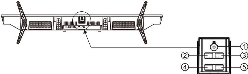
1. **POWER(⏻)/OK:** In the off mode, Short press to turn on the TV. In the on mode, Short press to achieve OK function, long press to achieve POWER function.
