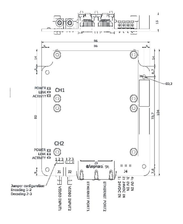
Figure 1 – Dimension and pin configuration.
