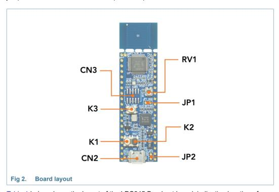
$\underline{\text{Table 1}}$  below shows the layout of the LPC845 Breakout board, indicating location of jumpers, buttons, connectors/expansion options and MCU devices.
