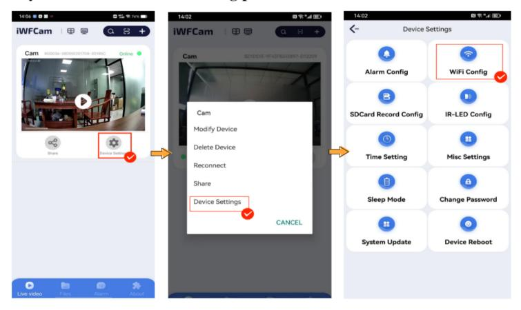
If the camera you purchased comes with the "sleep" function, After the camera is successfully connected to the network, it will automatically activate the sleep function when idle. Sleep mode can be turned on/off in the app. After turning off sleep mode, it has all the functions of a regular WiFi camera.
