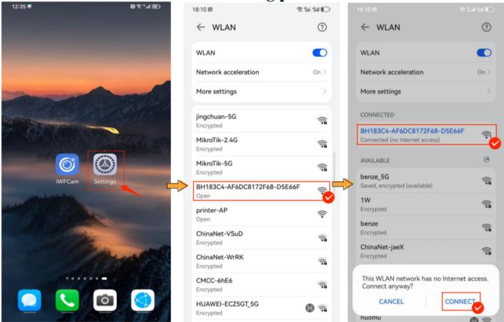
Step 3:Once your phone is connected to the camera's WiFi signal, open the "iWFCam" app, The camera will auto be added to the app and show "online". At this point, you will be able to view the camera's real-time video and control its settings.
