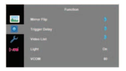
Function: press CAM2/> button enter into the function, press the CAM3/v or CAM4/^ button can select the Mirror Flip, Trigger Delay, Video list, light, VCOM.
