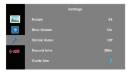
Rotate: this is rotate screen display mode, from 01 to 04 for choice.
