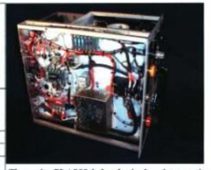
The entire PLA800 is hand wired, point to point to ensure solid contacts from component to component. With its heavy frame and solid construction, the PLA800 will give years of troublefree use.
