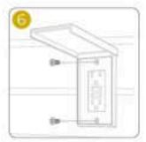
Use the provided stainless screws to attach the cover to the receptacle.
