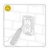
For irregular wall surfaces such as brick or stone, a bead of caulking (not included) may be used to seal the unit to the wall to prevent water intrusion.
