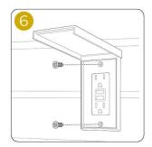
Use the provided stainless screws to attach the cover to the receptacle.
