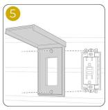
Place the cover over the receptacle and line up the mounting holes. The cover mounts to the outer set of holes on the receptical.
