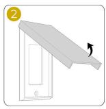
The cover is designed to be installed with the hinge at the top. Ensure the cover rotates upward during installation.
