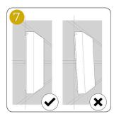
Ensure that the weather gasket is compressed consistently on the back of the cover creating a water tight seal. Do not over tighten the screws.
