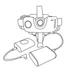
Once new battery lights up, unplug old battery and remove from battery mount
