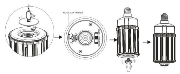
It could be easily installed using a straight screwdriver. Use a flat-blade screwdriver to unscrew the plug and removethe plug. And then. Choose motion sensor to install and tighten.
