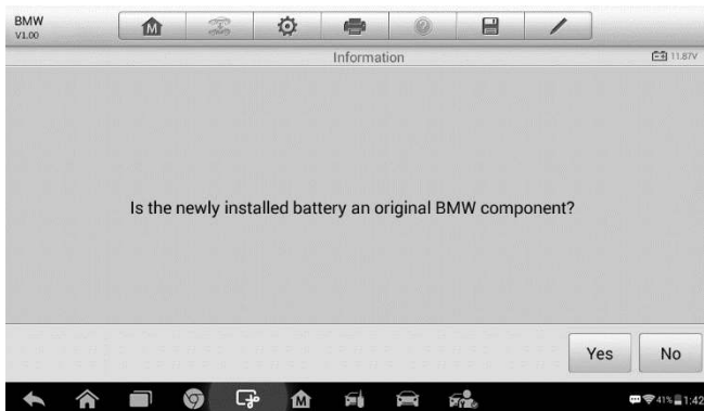
Figure 7-15 Sample BMS Screen 6
