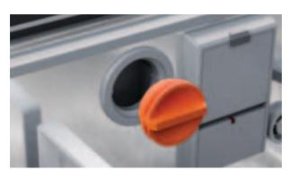
**3.** Remove the funnel and refit the cap, turning clockwise until secure.
