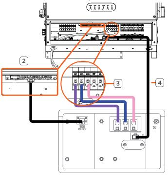
5. Make all connections between the inverter and the electrical system. Generator, and Load connections. For more information, see the Savant Power Storage 20 Deployment Guide.
