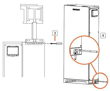
5. Install the bracket on the wall with M6x50 tapping screws.
