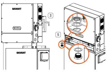
Gently plug in each battery module from the bottom up. Fasten the modules on both sides using M4x8 screws (Torque: 1.2 N·m).
