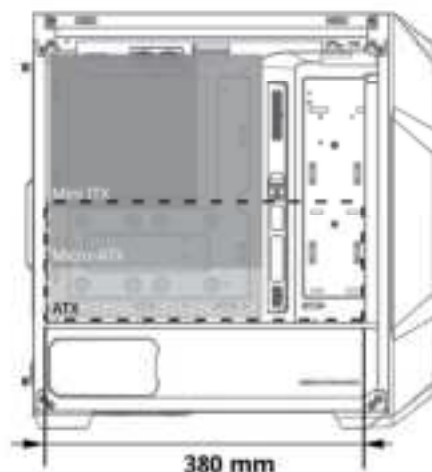
Maximum length for graphics card ( With pre-installed AIO on front )
