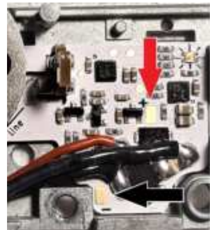
Tracer or mag terminals soldering pads
