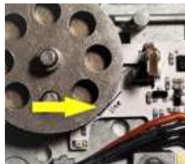
Sensor line and sector gear alignment
