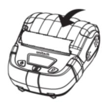
4. Tear off the excessive paper according to the direction as shown in the figure.
